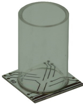
Figure 1: Electrochemical sensor with cell culture area (in transparent plastic cylinder).
