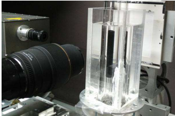
Figure 1. A photograph of the test section of the annular channel with the immersion unit filled with distilled water. Fragments of the laser head and camera lens are also visible in the picture, which displays the arrangement of the measurement system.
