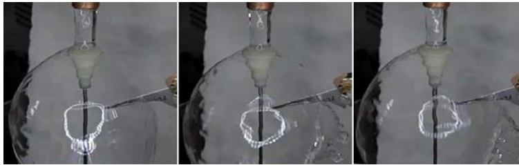
Figure 5. Patterns of the dome-shaped film, when the plate wide side is located along the flow velocity vector. On the left - wave regime, in the centre - discontinuity, on the right - coalescence. Flow rate is Q = 73 ml/s; U_0 = 1.2 m/s.
