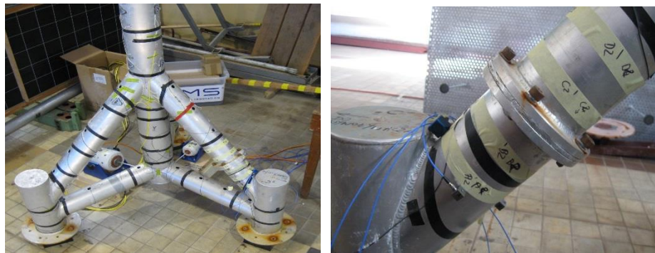
Figure 1. Laboratory scale model of the tripod supporting structure (left) and detail of the flange (right) used in order to simulate the propagation of the circumferential representative crack in the cylindrical brace.
