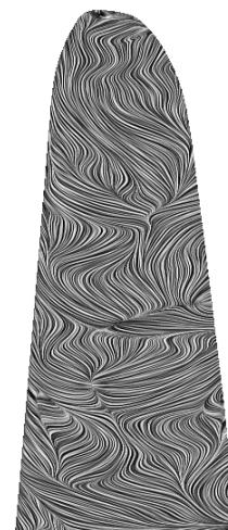
Figure 12. Instantaneous direction of wall shear stress on suction side near blade tip. Inflow speed: 40m/s, physical time: 20s.
