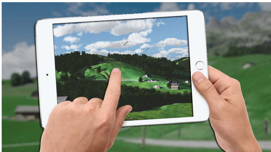
Figure 8. Assessment of a wind farm layout on site by augmented reality
