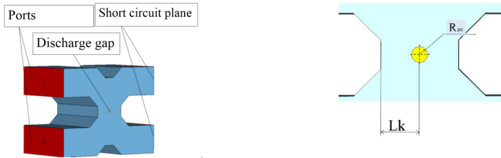
Fig.7. Joint phase shifting module with conductive cylinder for plasma column imitation.
