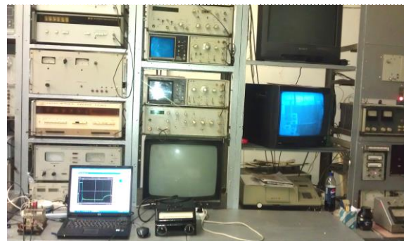
Figure 6. Control equipment for precise modification of high voltage thyristors.
