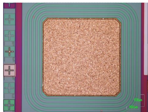
Figure 4. Appearance of pulse diode structure (3A, 200V) with guard rings
