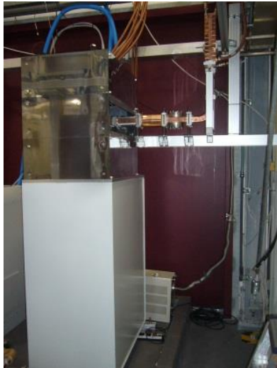
Figure 1. Modulator with klystron and local shielding.
