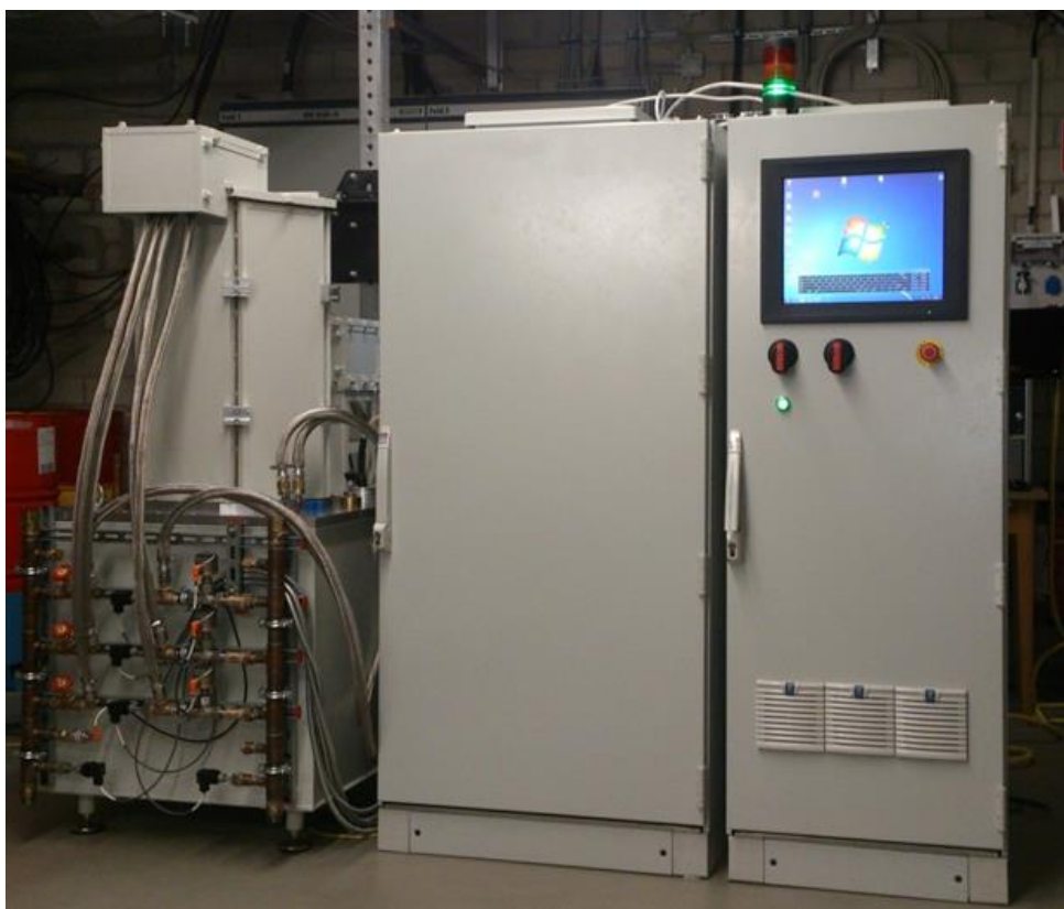
Figure 7. Klystron power supply XFEL TDS INJ: left – pulse transformer in oil tank with klystron and local shielding on the top; middle – modulator; right – control unit in power supply cabinet.
