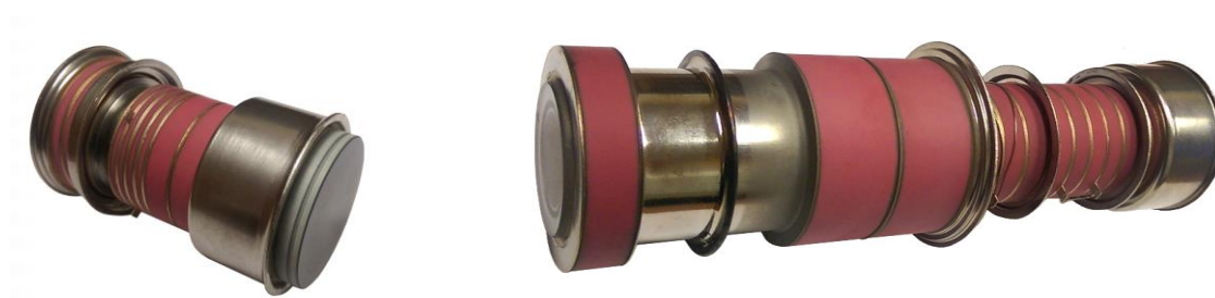
Figure 3. New generation streak tubes: TPO29 series (left) and TPO30 series (right).
