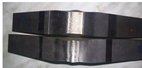
Figure 9. Welded joint after bending. Top sample - face, lower sample - flip side.
