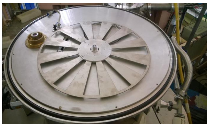
Figure 2. Rotors for the Fourier chopper.
