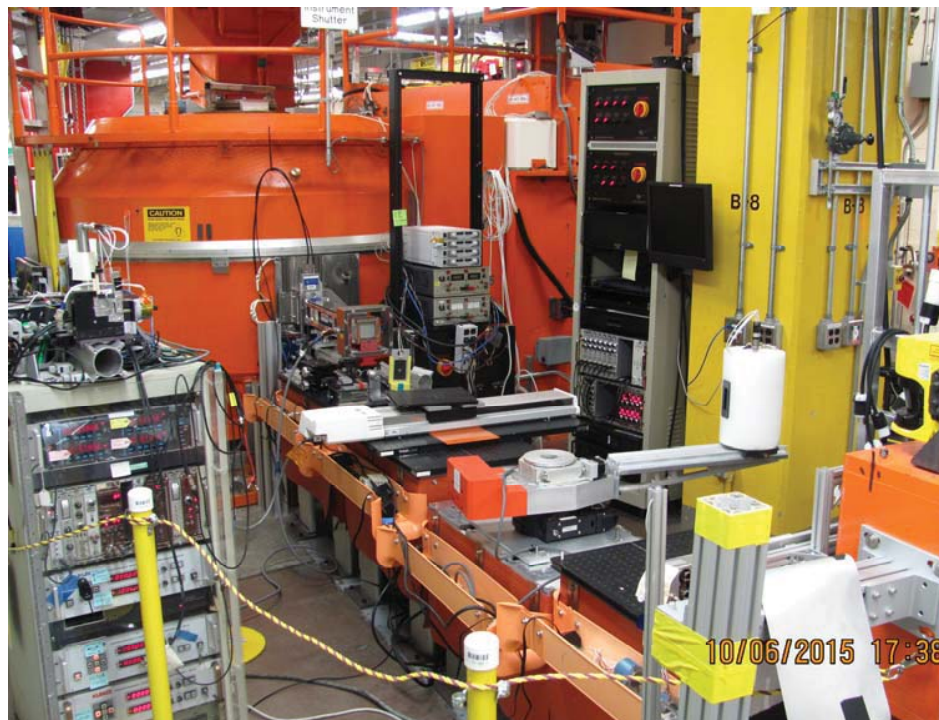
Figure 1. This figure shows the HB-2D monochromator drum (upper left), and the variable height lift tables between the exit port and the beamstop.
