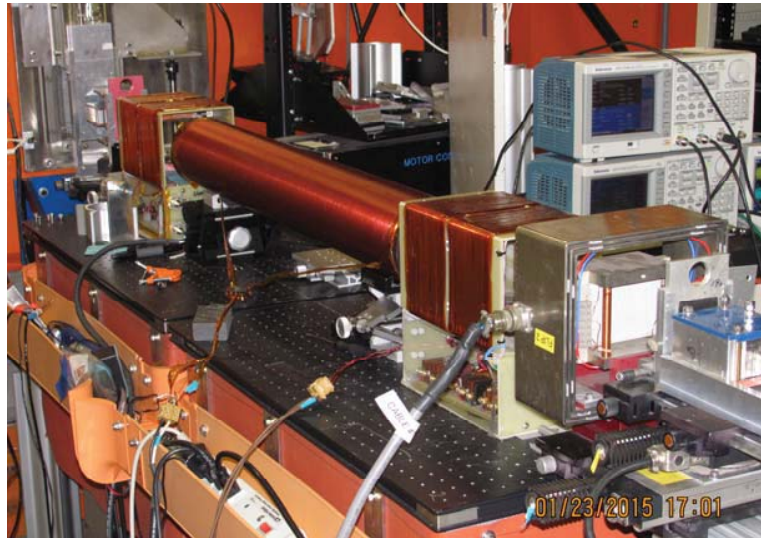
Figure 3. The Modulated Intensity by Combined Effort system is shown in its initial configuration. The square coils before and after the cylindrical solenoid are rf flippers. The solenoid current is varied to conduct a scan. A neutron detector downstream detects neutrons in time-of-flight, with the time base synchronized to the coils.
