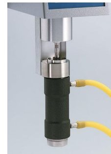
Figure 3. LVDV-II+Pro viscometer (UL adapter).
