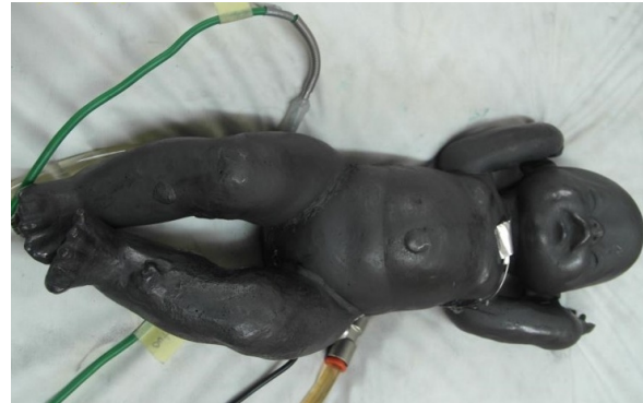
Figure 6. Thermal manikin lying on the mattress of radiant warmer bed. Visible water ports and thermocouples measuring surface temperature protected with aluminium foil.
