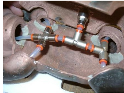
Figure 2. Stabilized temperature water delivery system.
