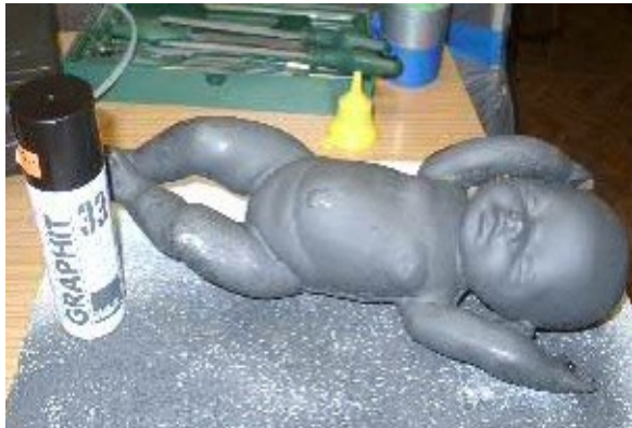
Figure 5. Thermal manikin covered with graphite (high emissivity) spray coating.
