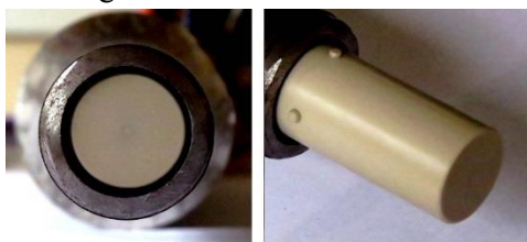
Figure 2. Cylindrical insert used as cross-sectional area reducer.
