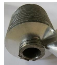
Figure 3. Sample of the tested finned tube. The fins density is 10 fpi here.
