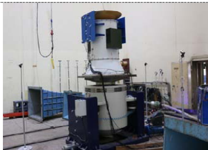
Figure 3. Vibro-acoustic test system of complex structure.
