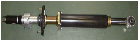
Figure1 Electromagnetic damper (2 nd prototype)
