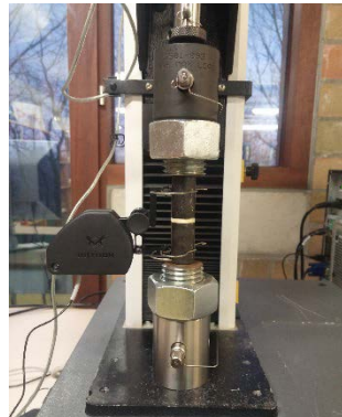
Figure 3. test setup for the quasi-static tests.
