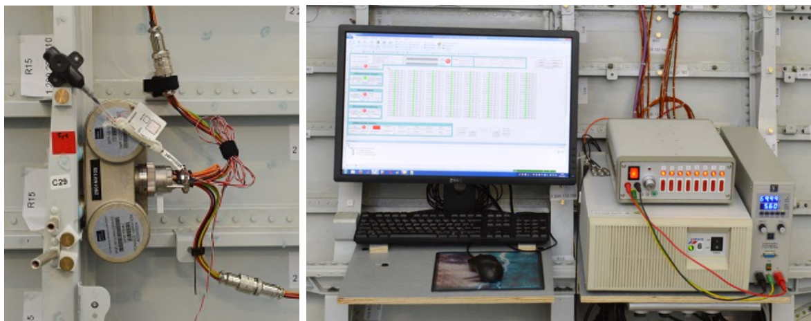
Figure 11. Detail view of one TVA (left), TVA system controls inside the fuselage (right)
