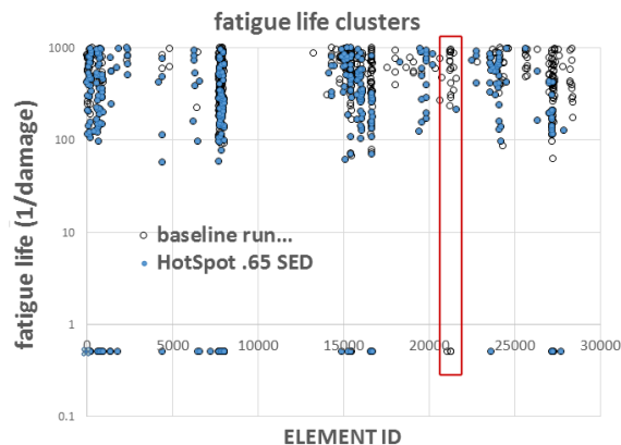
Figure 11 fatigue life for top damaged elements represented in order of element ID. Boxed area points to missed hotspots.
