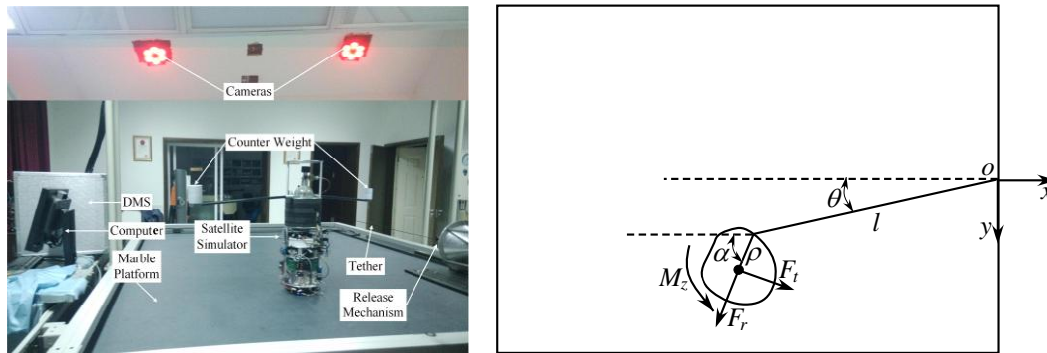
Figure 4. The experimental system and its mechanics model.
