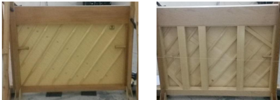
Figure 2. Laminated soundboard (left) and Tone-wood soundboard (right).
