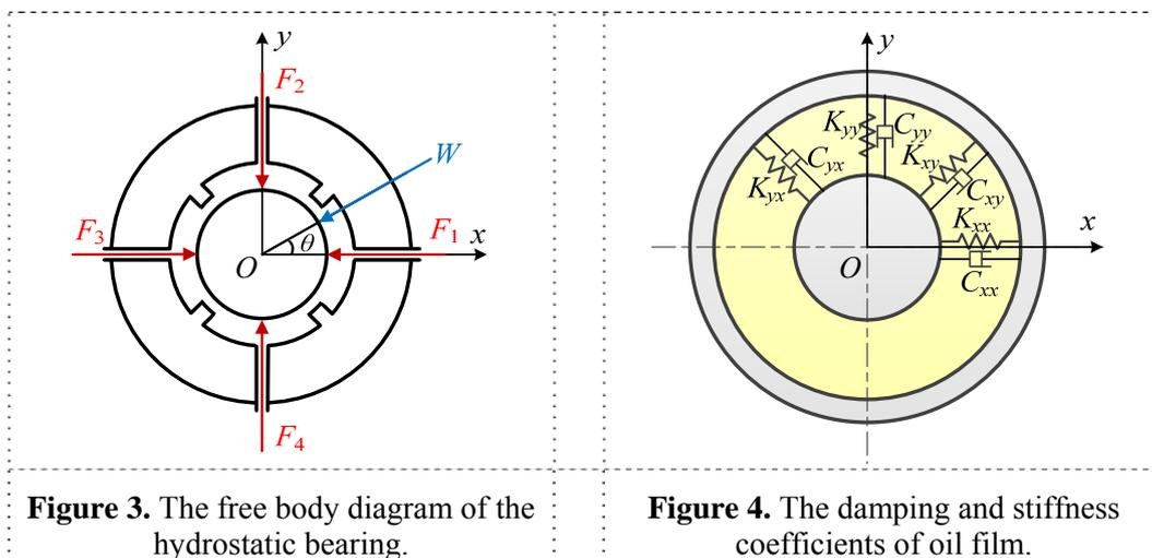
**Figure 3.** The free body diagram of the hydrostatic bearing.
