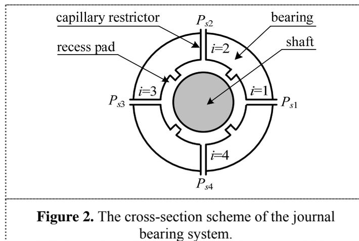
**Figure 2.** The cross-section scheme of the journal bearing system.
