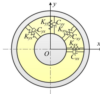
**Figure 4.** The damping and stiffness coefficients of oil film.
