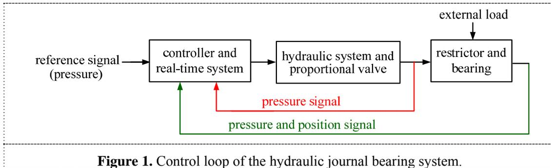
**Figure 1.** Control loop of the hydraulic journal bearing system.
