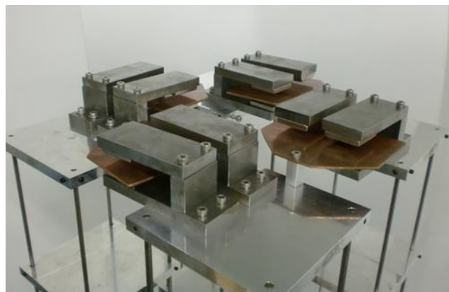
Fig.10 Outlook of four substructures with eight dampers
