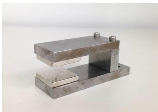
Fig. 4 Magnet for damper
