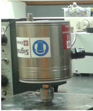
Figure 2: Experimental set-up of the inertial actuator “Data Physics IV40” fixed on the test-rig through a force cell with an accelerometer mounted on the moving part.
