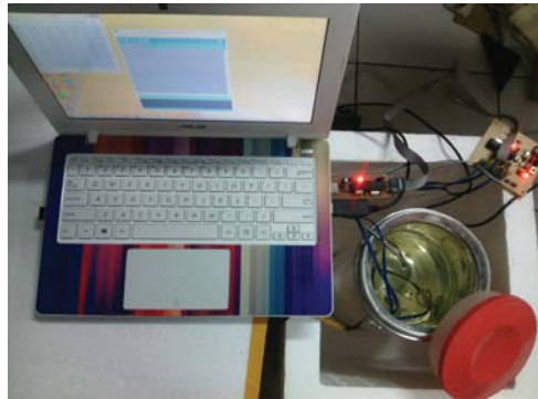
Figure 2. Photograph of the experimental setup for measuring the effectiveness of water as the sensible TES as well as CO and \text{CaCl}_2 \cdot 6\text{H}_2\text{O} as the latent TES.
