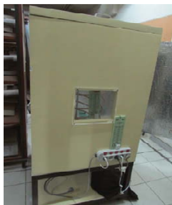
Figure 2. Thermal chamber and testing the CO as temperature controller.
