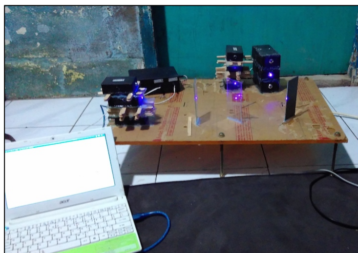
Figure 2. Experimental Equipment for Laser Pointer with Wavelength 405 nm.
