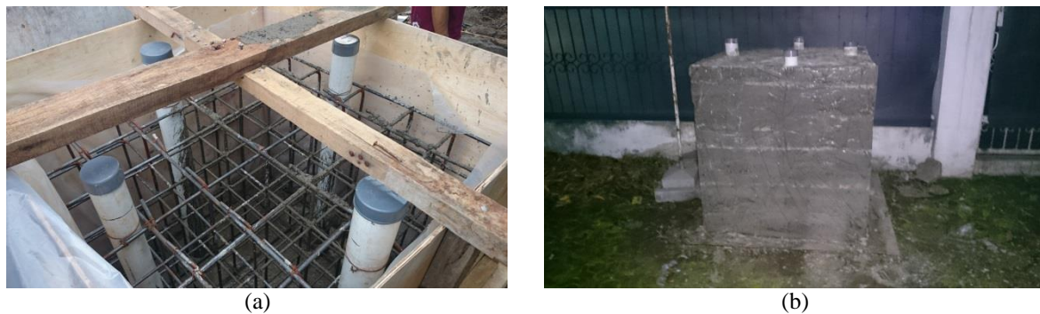
FIGURE 3. Bored pile model, (a) Before casting, (b) After casting
