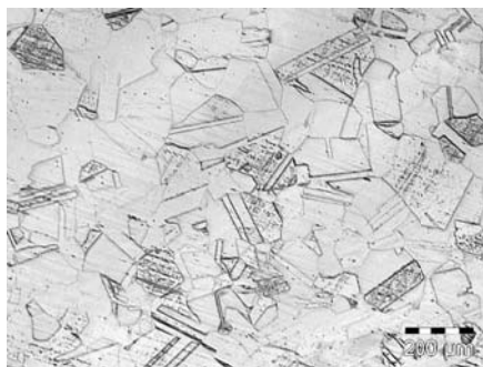
Figure 1. Microstructure of the cold rolled 304 stainless steel used in this study
