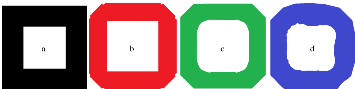
Figure 2. Simulated shapes under examination, with average lateral dimensions of 400 nm x 400 nm x 10 nm.
