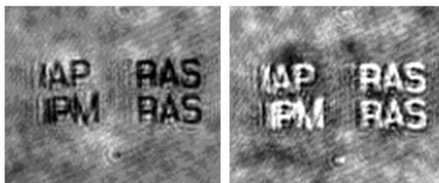
Figure 5. Direct and inverted microimages of the name of the institutions. Letter size 30 \mu\text{m} .
