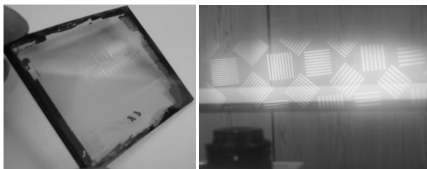
Figure 5. The experimental sample of the light guide substrate with a combination of DOEs and image of the test-object
