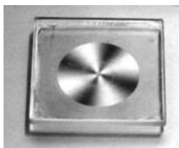
Figure 4 The photo of LC film with radial director orientation in-between cross linear polarizers
