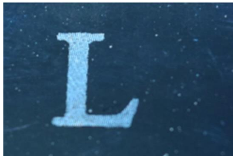
Figure 3. Direct laser recording on the a-Si layer of the interference filter by Blu Ray laser with a \lambda = 405 nm.
