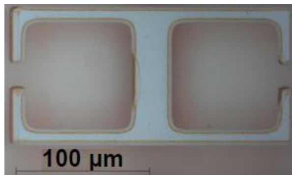
Figure 6. Microimage of fabricated MA sample with set of parameters: a=208\mu\text{m} , b=98\mu\text{m} , p=13\mu\text{m} , g=23\mu\text{m} , w=6\mu\text{m} .
