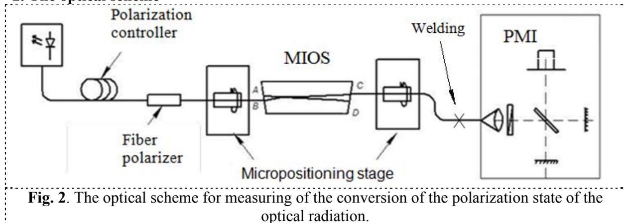
Fig. 2. The optical scheme for measuring of the conversion of the polarization state of the optical radiation.
