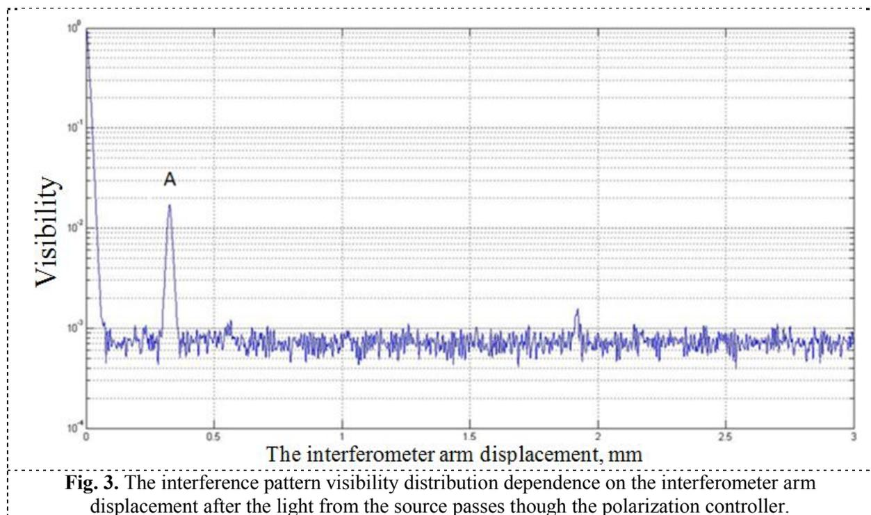
In fig. 3 point A - parasite interferometer peak from the radiation source.
