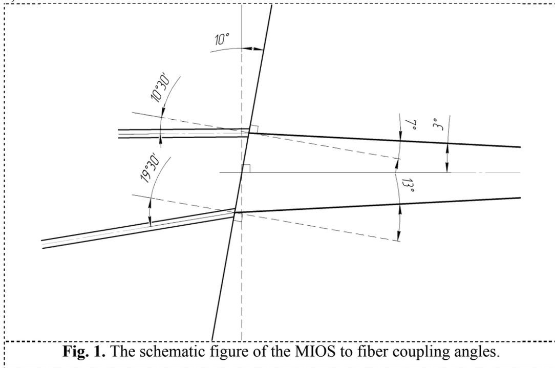
Fig. 1. The schematic figure of the MIOS to fiber coupling angles.
