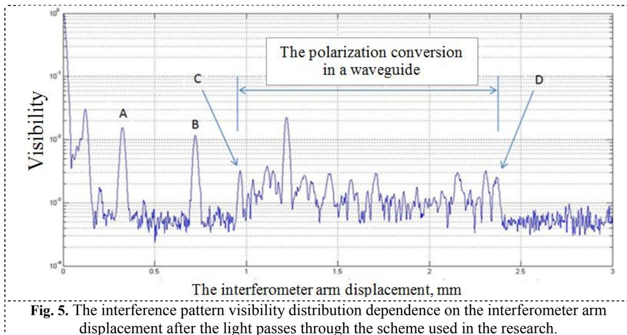
**Fig. 5.** The interference pattern visibility distribution dependence on the interferometer arm displacement after the light passes through the scheme used in the research.
