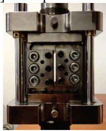
Figure 1. Simple shear device for AHSS
