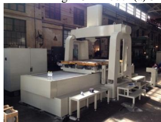
Fig.3-Incremental forming machine
