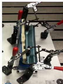
Figure 7. Stamped part on the checking fixture
