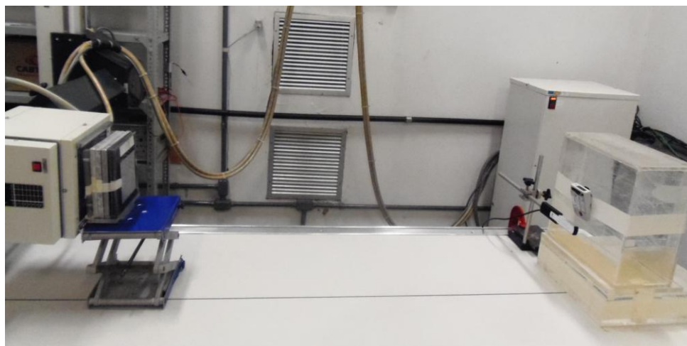
Figure 2 - Irradiation set-up for testing the electronic personal dosimeters in pulsed X-rays of a medical machine.
