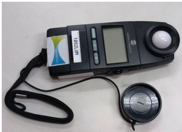
Figure 1. Photometer used in the comparison as comparison equipment.
