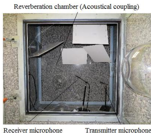
Figure 4. Experimental arrangement for diffuse-field reciprocity calibration in Inmetro.
