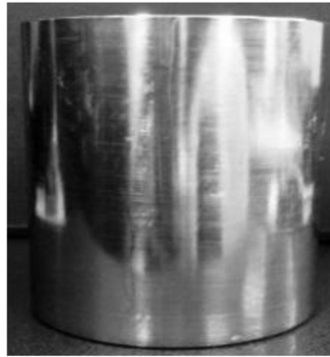
Figure 1. Stainless steel AISI 304 test body.
