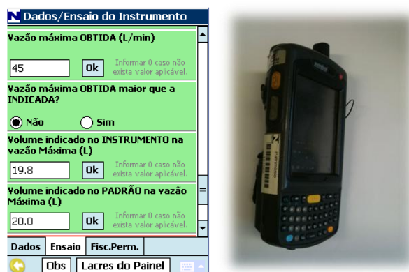
Figure 1. Data collector connected to IMS database used to perform metrological tests.
