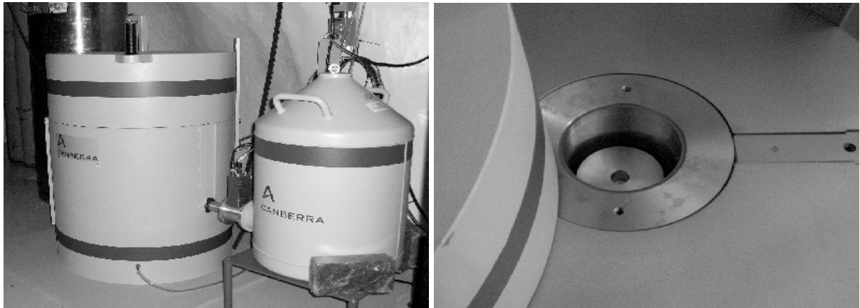
Figure 3. The SNOLAB Canberra germanium well counter. The right hand photo shows the detector and sample chamber.
