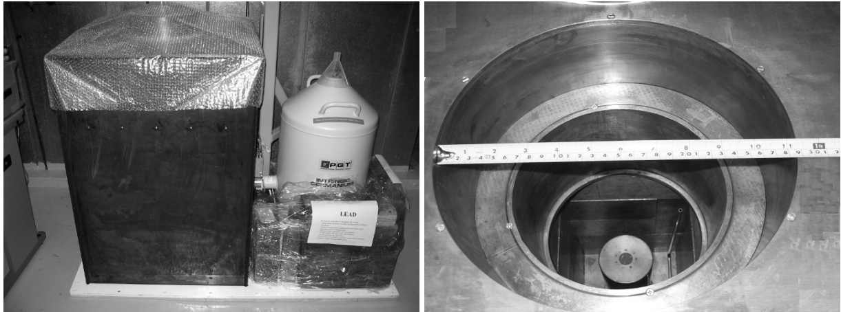
Figure 1. The SNOLAB PGT germanium counter, the copper box is used to seal the shielding to keep out radon. The right hand photo shows the detector and sample chamber.
