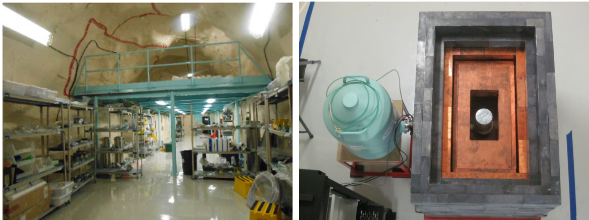
Figure 5. The top schematic shows the SNOLAB low background counting lab layout. The bottom left photo shows the current state of the low background lab and the right photo shows the Vue des Alpes germanium detector with its shielding partially in place
