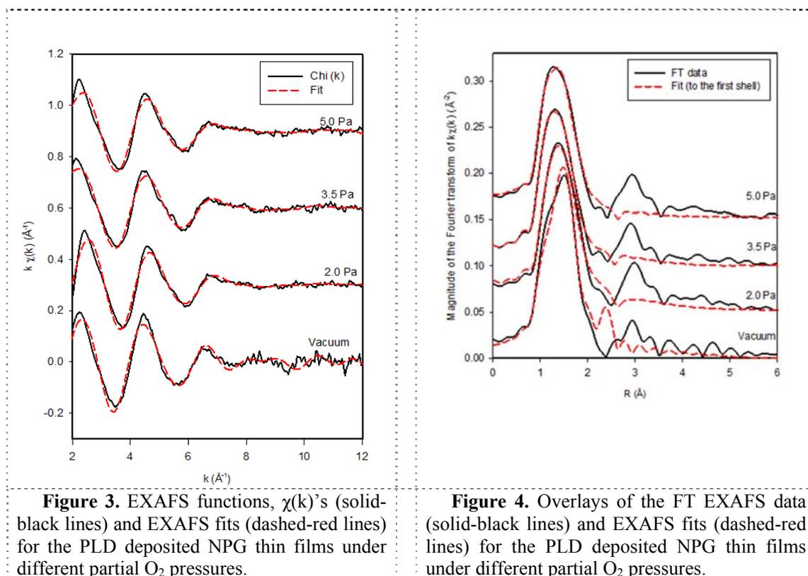
**Figure 3.** EXAFS functions,  $\chi(k)$ 's (solid-black lines) and EXAFS fits (dashed-red lines) for the PLD deposited NPG thin films under different partial  $\text{O}_2$  pressures.
