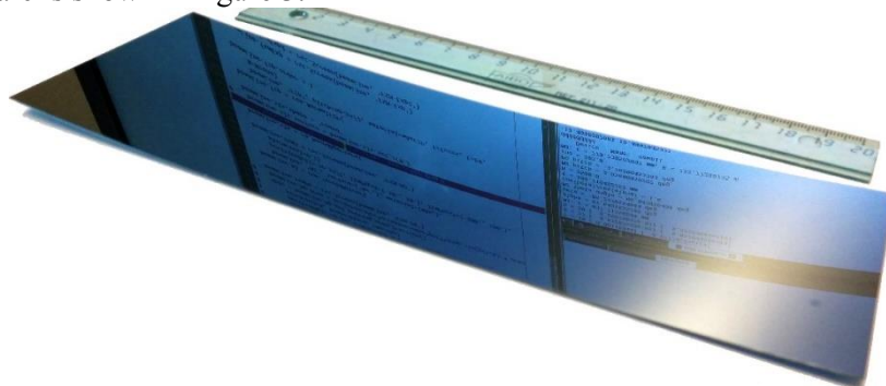
Figure 3. A ground and polished test silicon crystal. Notice that this is not a bent piece; the crystal planes are still flat and parallel to the table.
