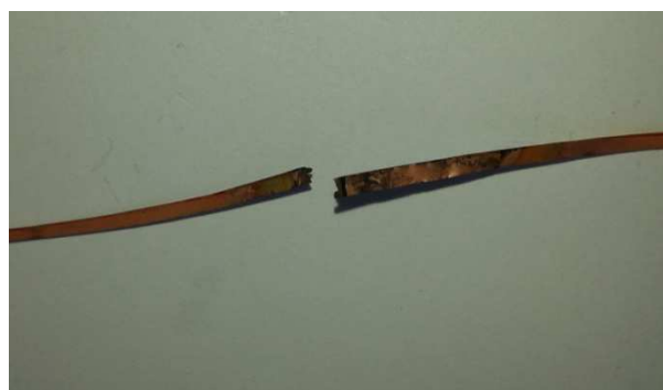
Figure 1. 2G superconducting tape burned out due to developed normal zone, initiated by thermal disturbance.
